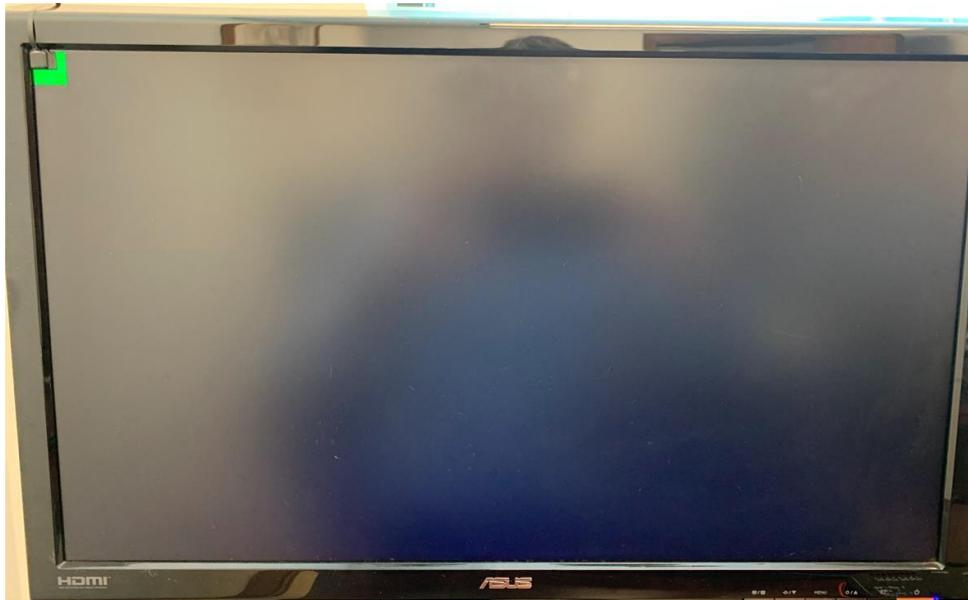
3. Use the Port 2 push button to size the green square appropriately. Press and Release Port 2 button until the green square is just hidden beneath the sensor housing. The green square should not be visible when standing in a normal viewing position in front of the screen.
