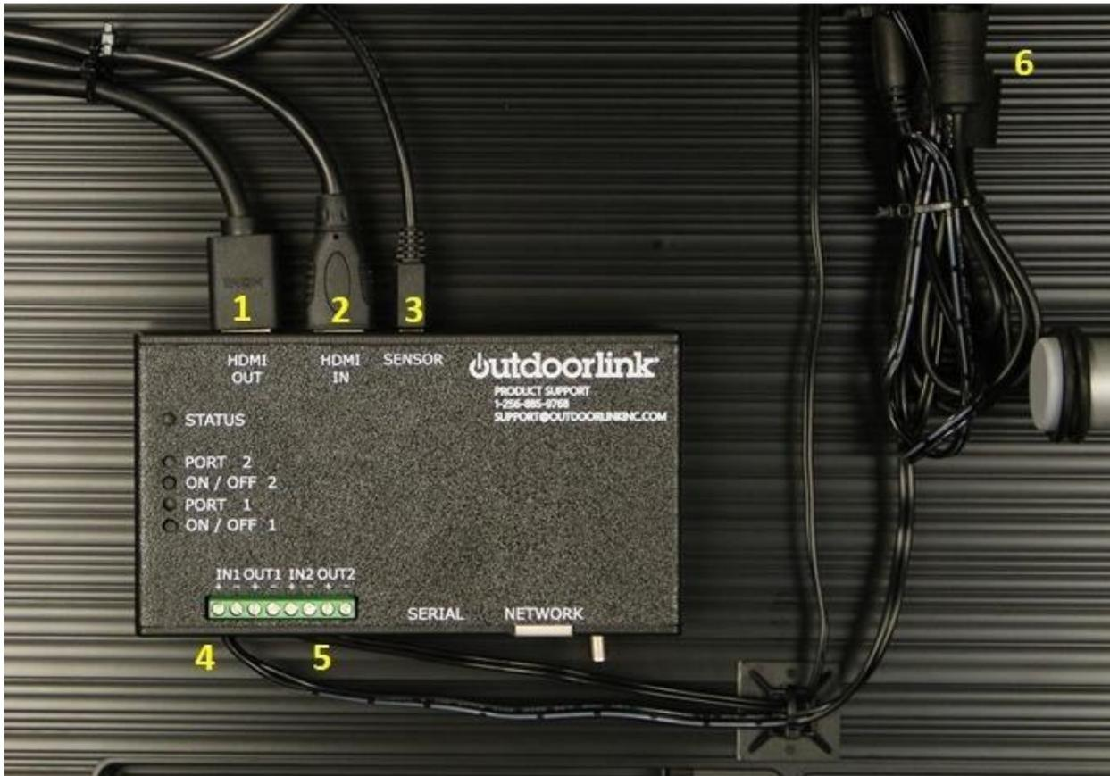
1. HDMI Out – Video Signal from Vantage Controller to LCD Display
