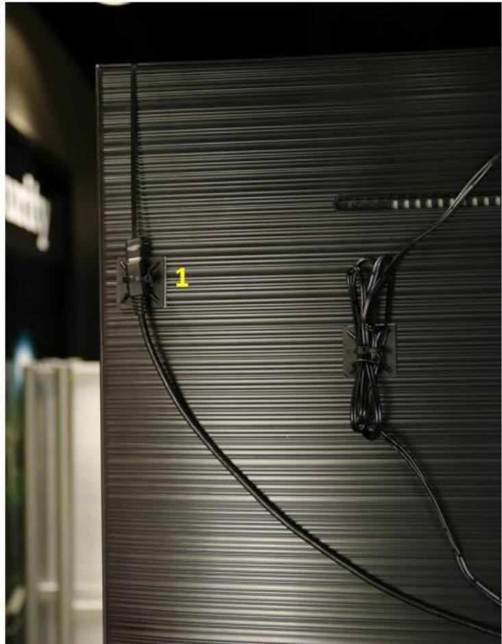
1. Flex Circuit Connector to Sensor Cable. Sensor Cable connects to Vantage Controller at “Sensor” interface. This port is labeled on the enclosure.
